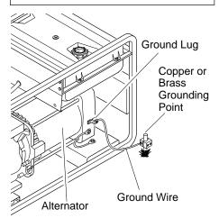
Figure 13 - Grounding Generator (Model PGH7500IE Shown)
